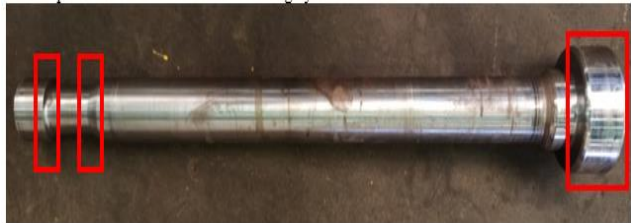
Figure 8. The positions of fillet in the tie rod shaft.
