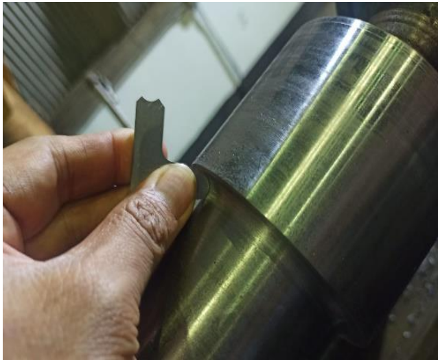
Figure 9. The measurement using fillet gauge.
