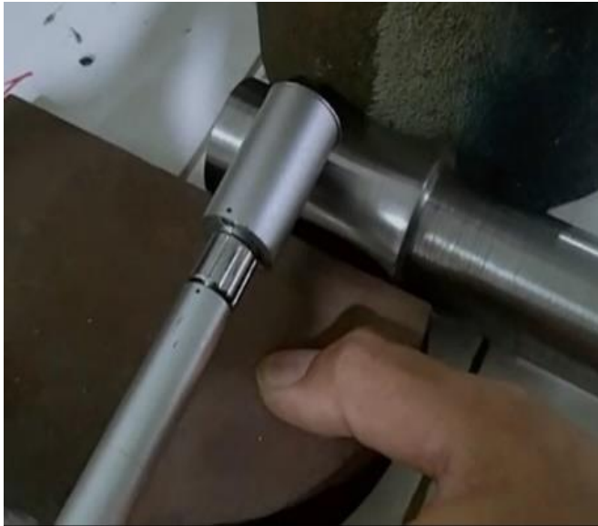
Figure 10. The surface roughness measurement.
