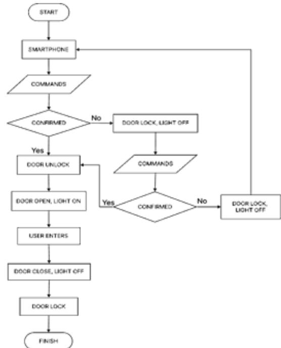
Figure 1. Flowchart of Automatic Sliding Door and Light Using NodeMCU Sensor.
