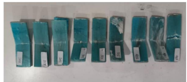
Figure 7. Bending specimen after testing
