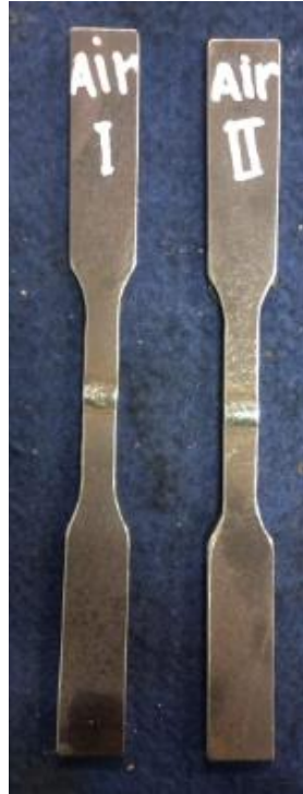
Figure 3. Tensile test workpiece according to ASTM E8 standard
