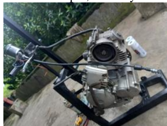
Figure 10 Yamaha Scorpio Engine
