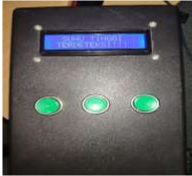
Figure 9. Display of The Tool When detecting excessive temperature
