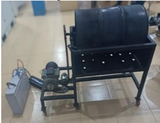
Figure 2.1 Automatic coffee roaster with a capacity of 20 KG with an AC motor
