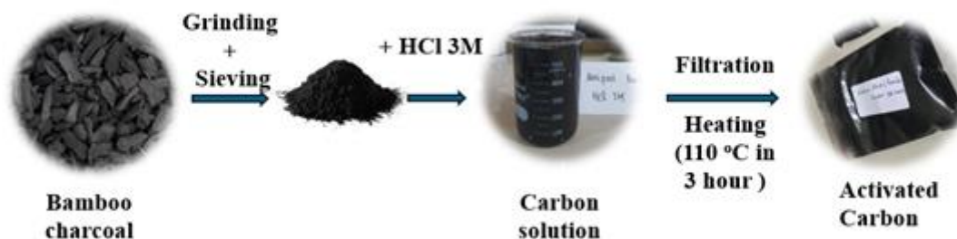
Figure 1. synthesis proses of Activated carbon from bamboo
