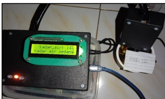
Figure 9. Display of 4-day drying results in room temperature
