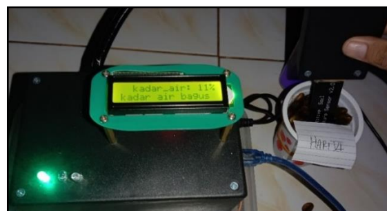
Figure 11. Display of 6-day drying results in room temperature
