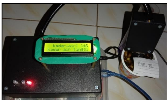
Figure 8. Display of 3-day drying results in room temperature
