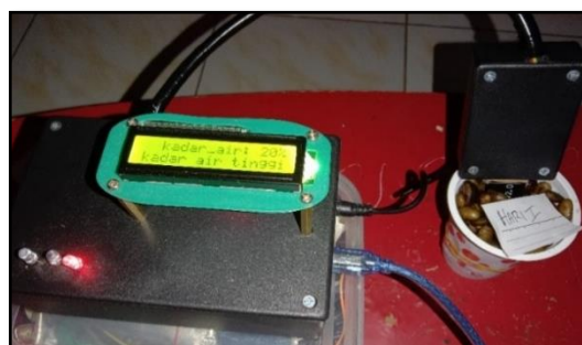
Figure 6. Display of 1-day drying results in room temperature
