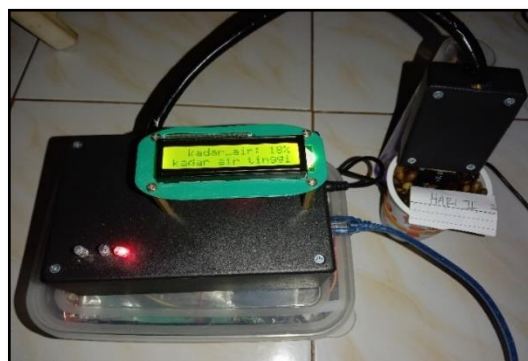
Figure 7. Display of 2-day drying results in room temperature
