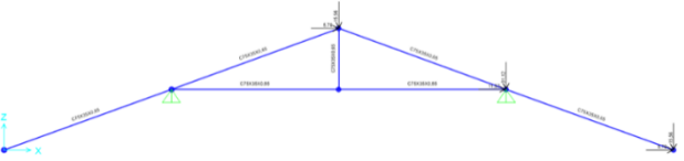
Figure 11. Wind Suction Load on Rear Trusses
