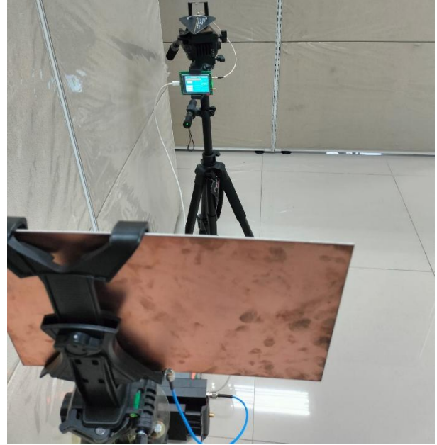
Figure 4. Antenna testing using a spectrum analyzer
