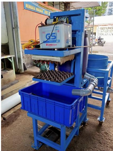
Figure 2. Prototype of the Paper Egg Tray Machine in operational condition, featuring the dual-power system, vacuum-assisted forming mold, and pulp collection container, assembled for functional testing in the campus environment.
